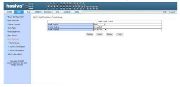
Figure 15 link aggregation configuration page
