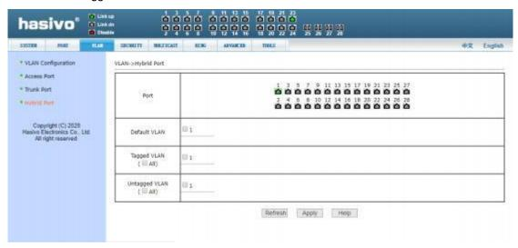
Figure 20 configuration page of hybrid port
