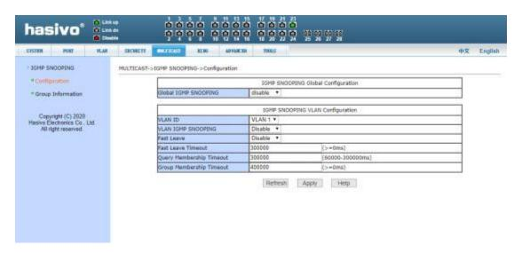
Figure 34 igmpssnooping configuration page
