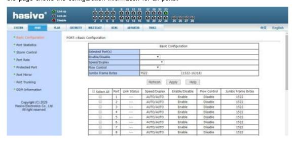
Figure 11 port configuration and port display page
