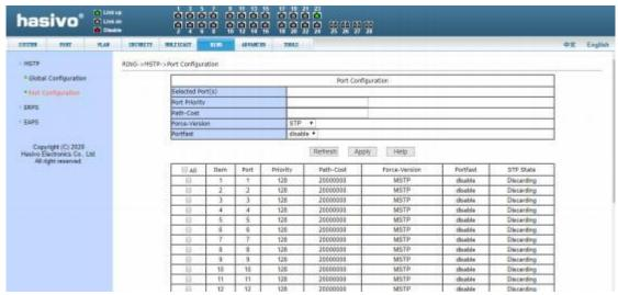
Figure 37 spanning tree port configuration page
