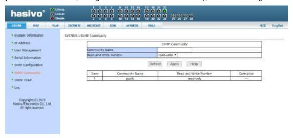
Figure 8 SNMP common configuration page
